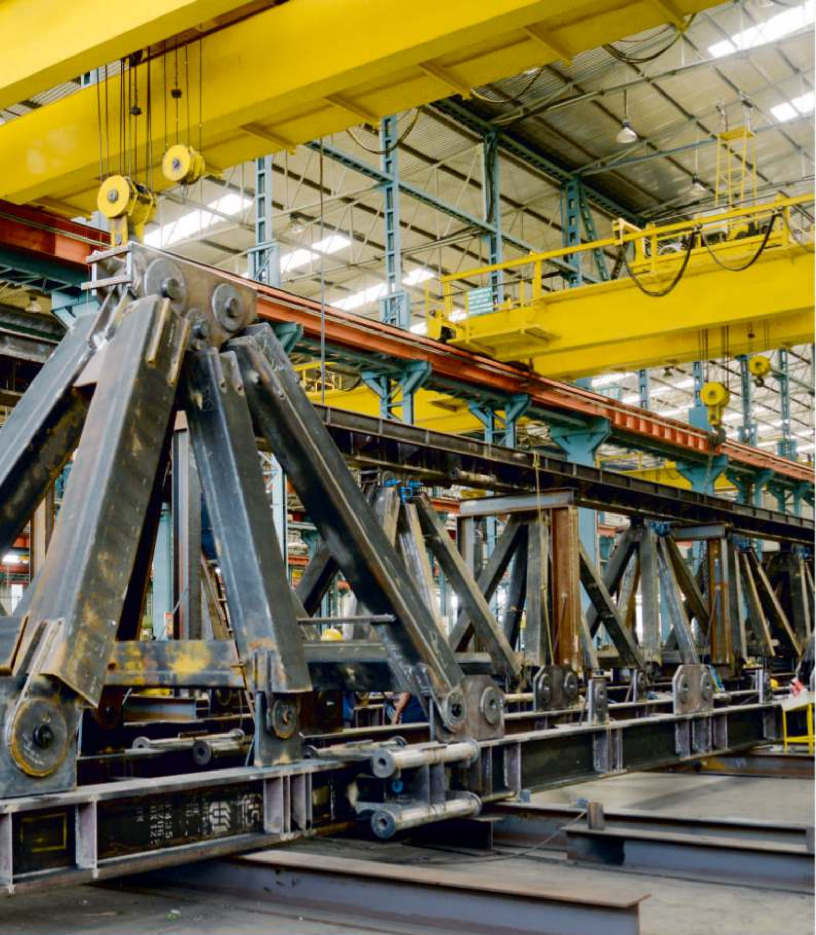
Fabricated steel gantry
