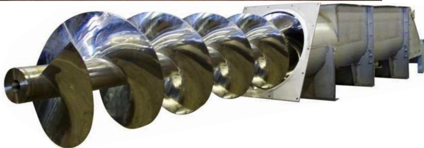
Shop assembly and trial of extra long 750MM dia SS screw conveyor
