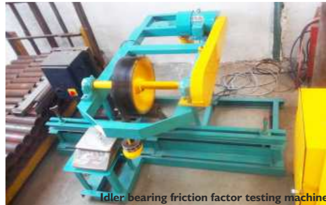
Idler bearing friction factor testing machine
